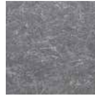
03 - Tumbled & De-burred Bare Material. No Protection
